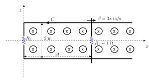
Moving bar in the presence of a constant magnetic field produces an emf and electric fields in the lab frame that drive a loop current I.
