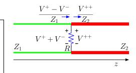
**Exercise:** Two TL's with characteristic impedances  $Z_1$  and  $Z_2$  are joined at a junction that also includes a series resistance R as shown in the margin. Determine the reflection coefficient  $\Gamma_{12}$  and transmission coefficient  $\tau_{12}$  at the junction.
