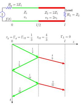
**Example 1:** In the circuit shown in the margin with two TL segments, line 2 has twice the characteristic impedance and propagation velocity of line 1, i.e.,
