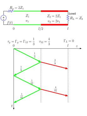
**Example 2:** In the circuit of Example 1, determine V(z,t) and I(z,t) if  $f(t) = \sin(2\pi t)u(t)$ ,  $t \text{ in } \mu s$ , and l = 2400 m,  $v_1 = 150 \text{ m}/\mu \text{s}$ , and  $Z_1 = 25 \Omega$ .
