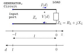
• In the TL circuit shown in the margin an arbitrary load  $Z_L$  is connected to a TL of length  $l = \frac{\lambda}{2}$  at the source frequency.
