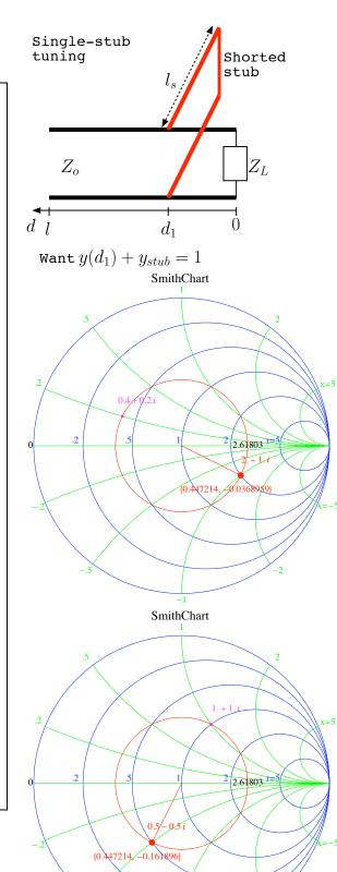
The required input impedance of the shorted stub to achieve
