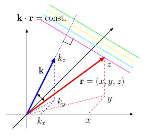
• In a homogeneous region where  $\epsilon$ ,  $\mu$ , and  $\sigma$  are, by definition, independent of  $\mathbf{r}$ , plane-wave solutions of phasor-form Maxwell's equations given in the margin become possible provided that
