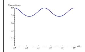
A plot of the transmittance  $1 - |\Gamma_{21}|^2$  versus  $d/\lambda_2$  is shown in the margin. The transmittance shows a  $\lambda_2/2$  periodicity in slab width d in consistency with the periodicity expected for lossless TL systems.
