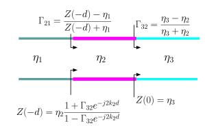
**Example 1:** Assume that regions 1 and 3 are free space whereas region 2 is a plasma slab of some width d and a plasma frequency  $f_p$ . Determine and plot the transmittance
