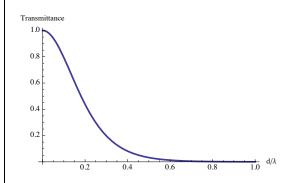
Note that adjusting  $d/\lambda$  to about 0.2 sets the transmittance as 1/2, creating in effect a "beam splitter" in reference to our discussions of prisms and tunneling in Lecture 24.
