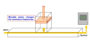
2. Dielectric filled cavities will have resonant frequencies
