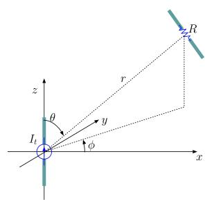
Current  $I_r$  that flows through the resistor R connected across the antenna terminals is induced by the tangential components of incident wave fields on the conducting arms of the dipole antenna; this response is a straightforward consequence of the need to maintain tangential boundary conditions on the antenna surface.
