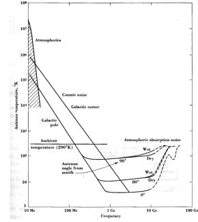
Antenna temperature curve from Kraus, "Radio Astronomy" (1966): Note that  $T_a$ is dominated by atmospheric noise (lightning, man-made noise) at low frequencies and by thermal emission from absorbing gases in the atmosphere past about a GHz. So-called cosmic noise from radio galaxies (including our own) dominates in VHF and UHF band.
